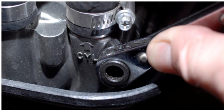
Figure 7. Ratcheting Box End Wrench. This tool provides rapid removal and installation with limited bolt head access.
