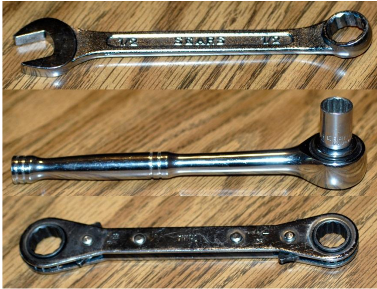
Figure 6 Box End, Ratchet, and Ratcheting Box End Wrenches. The ratcheting box end wrench is the result of applying Inventive Principle 5, or merging.
