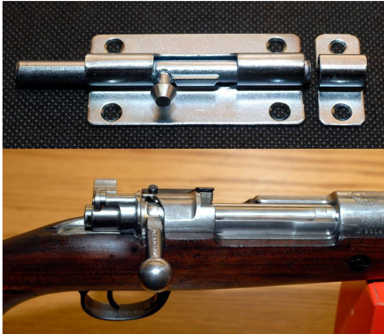
Figure 2. Bolt Mechanisms On Gate Latch and Mauser Rifle. A simple gate lock mechanism inspired the bolt action rifle.
